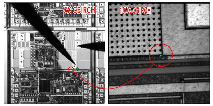
Rejected unit was used for investigation (the lot yielded poorly about 30%). OBIRCH clearly localized place where change of the resistance was marginal. In parallel investigation in PAL was on-going. The root cause found by PAL: incomplete removal of the polysilicon which caused a short to Metal1 in INV\_PWR\_PMOS. Detailed report is available only for internal purposes.
